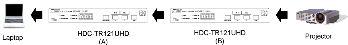
[Fig. 8.4] Reading EDID in daisy chain connection
