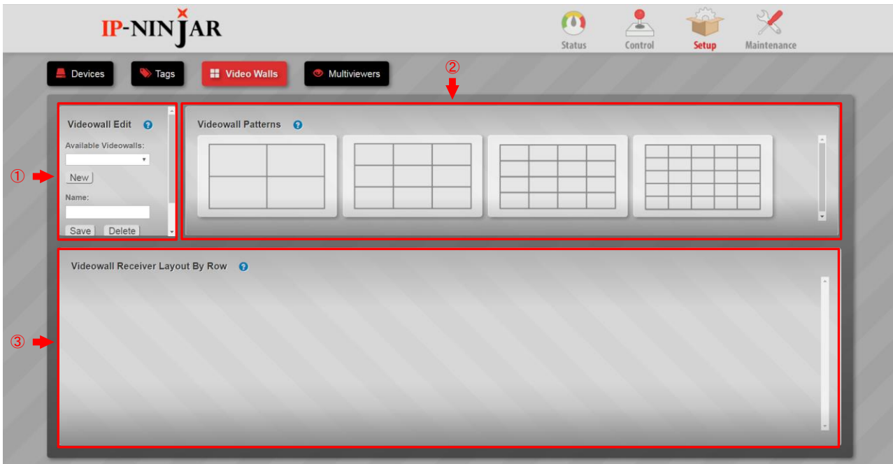
[Figure 10.15] Window for setting Videowall
