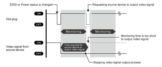
If the interval is shorter than the time for source device output video signal, the source device repeats the video output process and does not output video signal. This problem can be solved by setting longer monitoring time.
