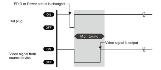
**Example:** The source device stops outputting video signals  $\rightarrow$  Hot plug request is needed.
