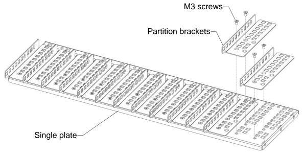
[Fig. 6] Removing partition brackets
