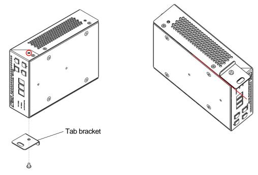
[Fig. 9] Attaching tab bracket
