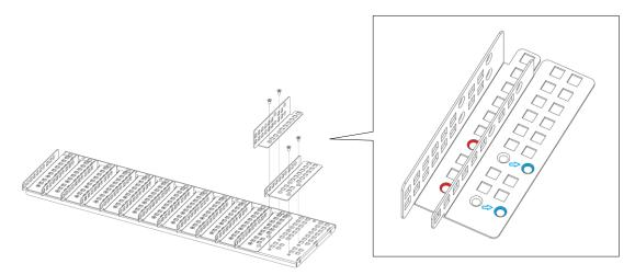
[Fig. 8] Attaching partition brackets
