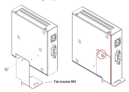
[Fig. 11] Attaching tab bracket BM
