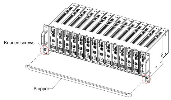
[Fig. 13] Attaching stopper bracket
