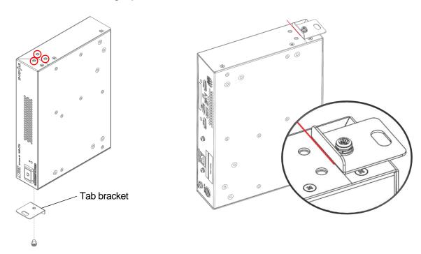
[Fig. 10] Attaching tab bracket
