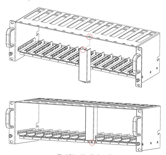
[Fig. 14] Attaching blank panel
