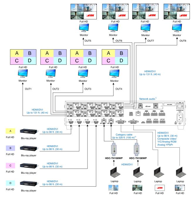
Up to 328 ft. (100 m): 4K@30 Up to 492 ft. (150 m): 1080p (24 bit) in Long reach mode For long reach mode, video signals up to 1080p (24 bit) can be transmitted to 492 ft. (150 m) at maximum
