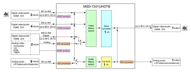
\*Maximum extension distance Up to 98 ft. (30 m): 1080p@60 Up to 39 ft. (12 m): 4K@60 (when 18 Gbps high-speed cable is used) (IN1, IN2, IN3 and OUT1 only)
