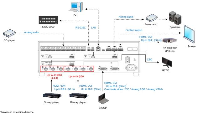
Up to 98 ft. (12 m): 4K@60 (when 18 Gbps high-speed cable is used) (IN1, IN2, IN3 and OUT1 only)
